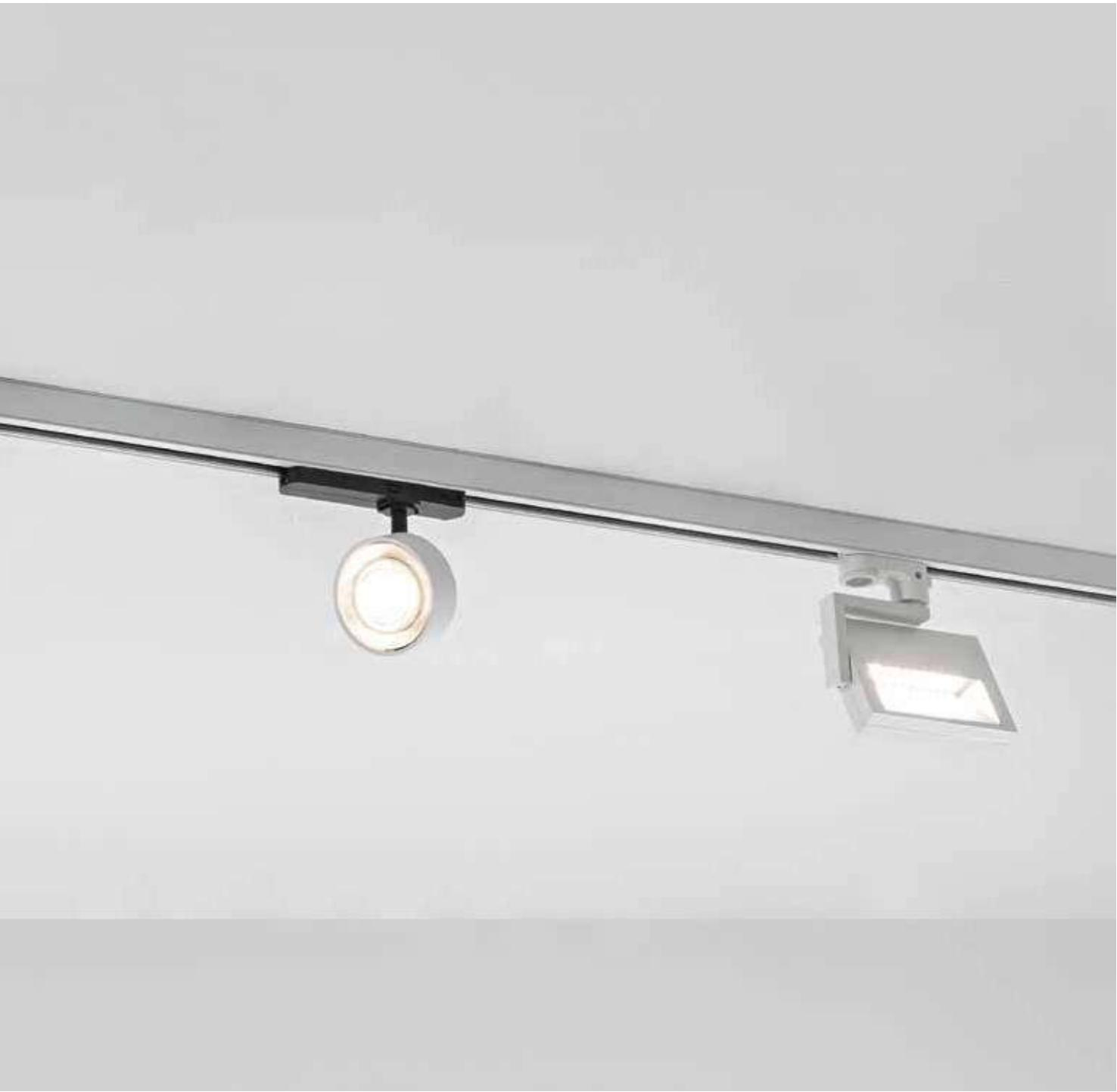
Three-phase and DALI track, 230V/440V-16A, with triple switching. Square section for wall, ceiling, suspended or recessed installation with appropriate accessories. Body in extruded aluminum alloy, copper wires housed in extruded PVC. Available in three sizes and three finishes (white, grey and black). Even in DALI version as system installation is possible with linear and angular joints.
